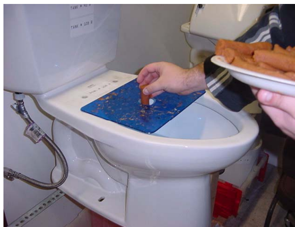
Test rig (top left), bulk & extruded media (top right), media (bottom left), and adding media to bowl (bottom right).
